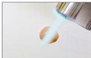
5. Provide a silicate layer with Pyrosil Gas
